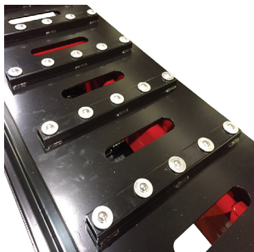
Open runway slots under rear slip plates
